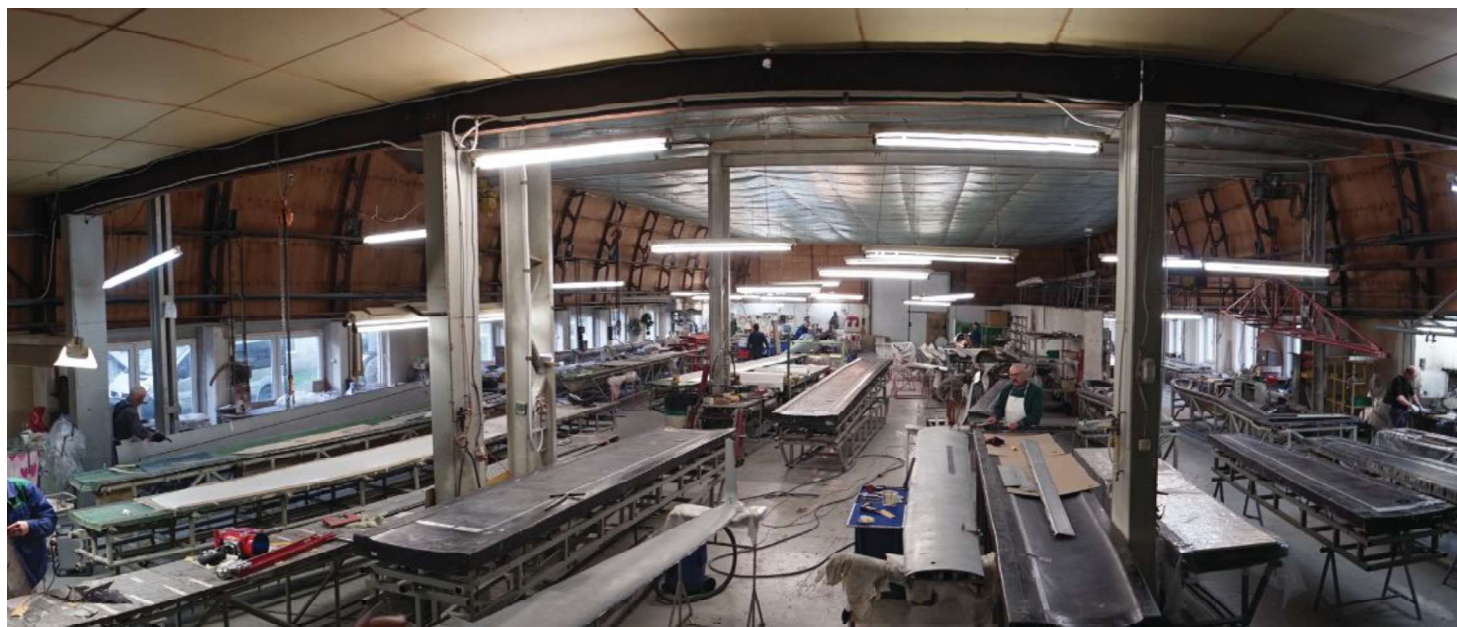
Factory floor showing spar molds. (Photo by Matt Herron.)
